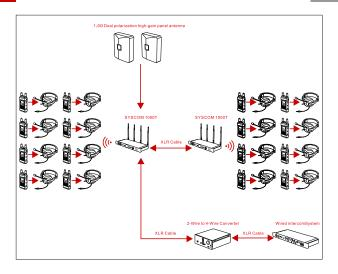
SYSCOM 1000T with standard 4-wire audio interface, which can connection with different type of intercom system to increase the quantity of beltpacks and also the wireless communication range. And if the live environment is complex, you can enhance the anti-interference by change the standard antennas to panel antennas.
